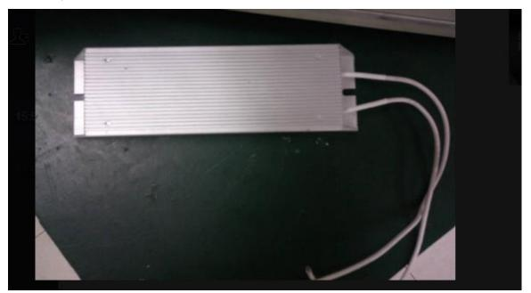
You need to remove the iron sheet or cable connecting P + and D on the drive and connect the two ends of the brake resistance to P + and C respectively. The corresponding parameters can be set by referring to the table below. for example:
